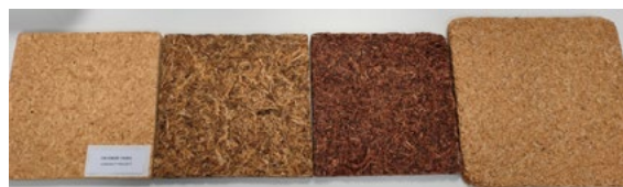
Figure 10. Experimental fiberboards developed from (left to right) fir (control), artichoke, vine shoot and rice husk fibers.
