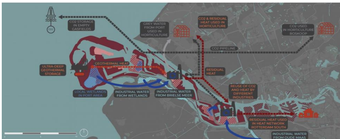
Figure 16. Flow of water and heat in the port of Rotterdam
